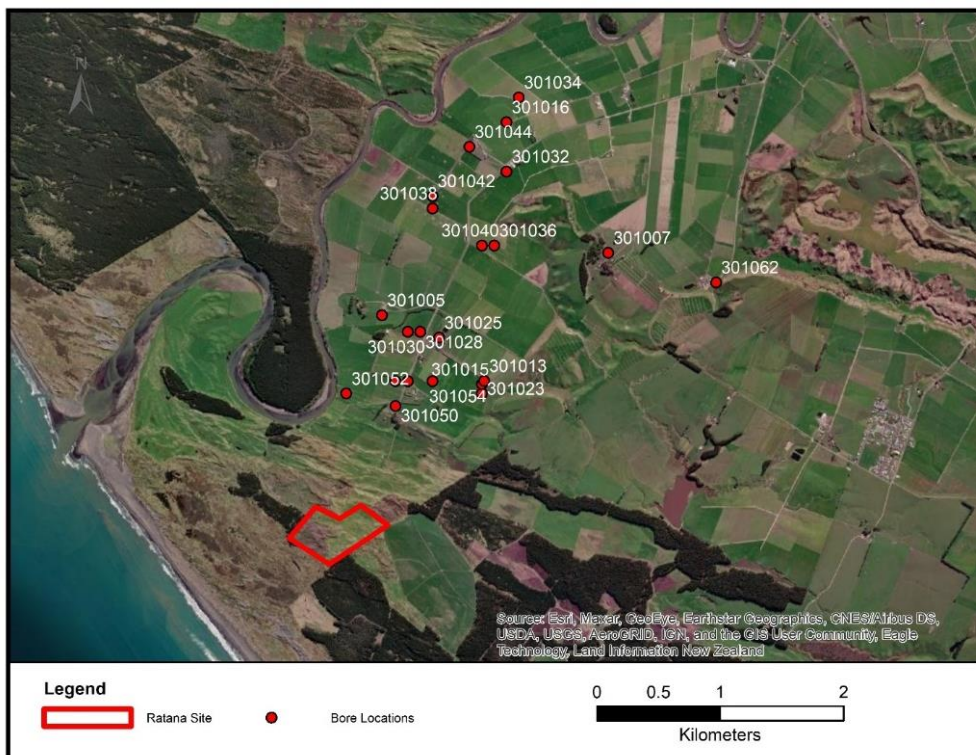
Figure 2-2: Bores within a 3 km radius of the proposed Rātana wastewater irrigation site.
